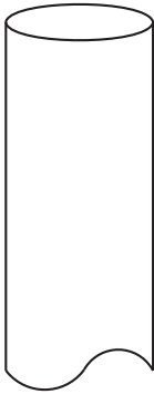
PVC Downpipe (DP65/80)
